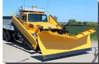
has a 300-gallon capacity for brine or other anti-icing and de-icing chemicals; and can pre-wet salt using pipes inside the bed before augering it to the spinner. The truck is a useful addition to SHA's fleet year-round. All the plows can be removed to convert the truck to a regular dump truck for hauling.
